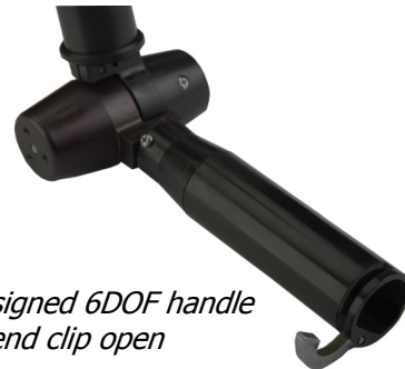
Pinch-capable PHANTOM 1.5 High Force/6DOF with thumb-pad end effector Note: Units now ship with chrome components**
